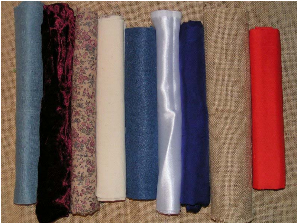
A variety of contemporary fabrics. From the left: evenweave cotton, velvet, printed cotton, calico, felt, satin, silk, hessian, polycotton.
