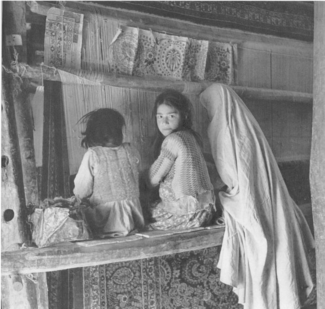
Girls weaving a Persian rug, Hamadan, circa 1922. Note the design templates ( called 'cartoons') at top of loom.
