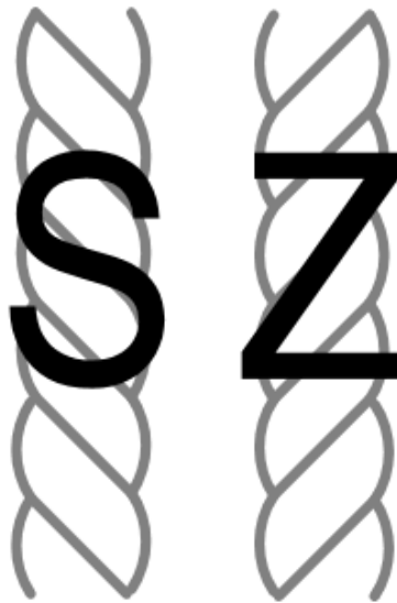
S-twist and Z-twist yarns
